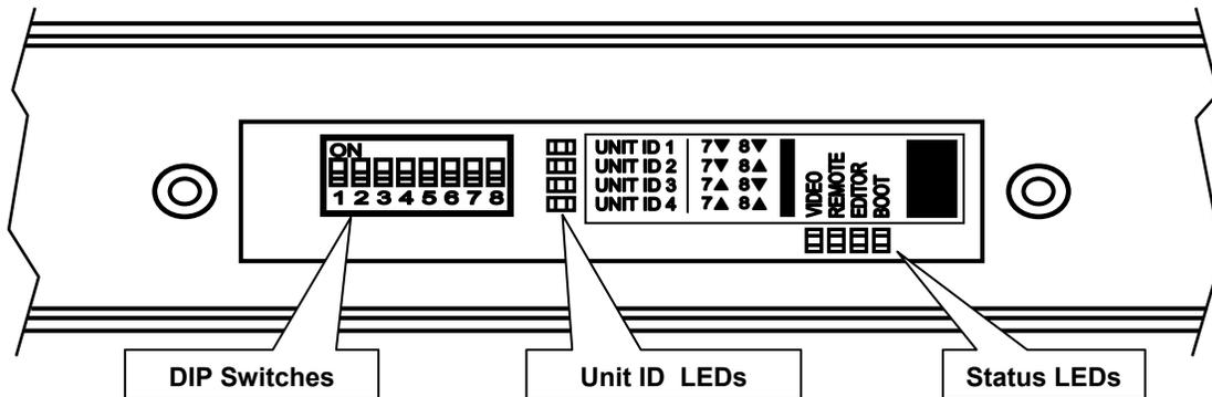
Figure 16.2.1. Main Unit Front View (Front Cover Removed)
