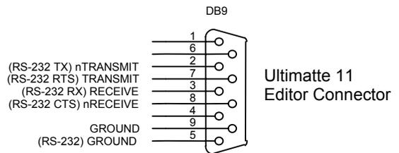
Figure 2.13.2. Rear Panel and Connector Pin Out
