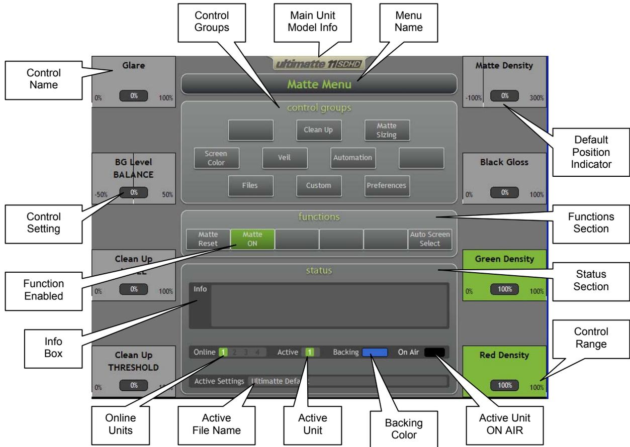
Figure 4.4.1. Smart Remote 2 Display
